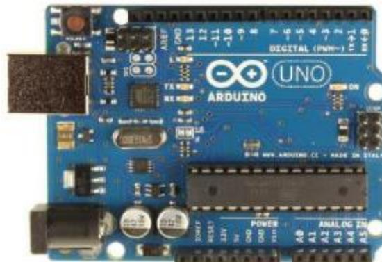
Gambar 2. Board Arduino Uno
