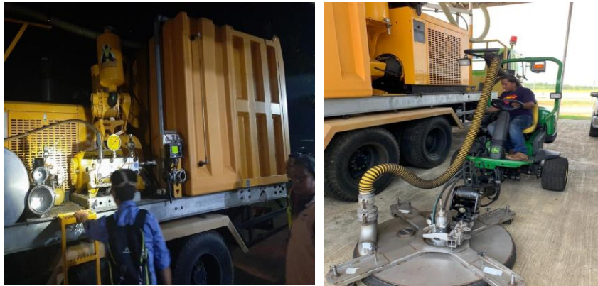
Gambar 4. Alat rubber deposit removal Water Blasting SK3000
