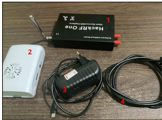
Figure 7. Receiver device, which consists of (1) Hack RF, (2) Raspberry Pi, (3) power supply adapter, and (4) USB communication cable.
