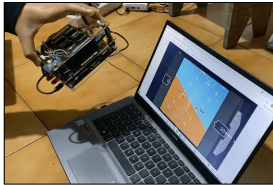
Figure 8. Primary Flight Display in action, receiving and visualizing real time data from the transmitter.
