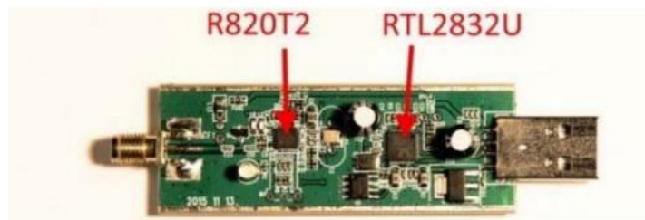
Gambar 3. RTL SDR R820T2 [3]
