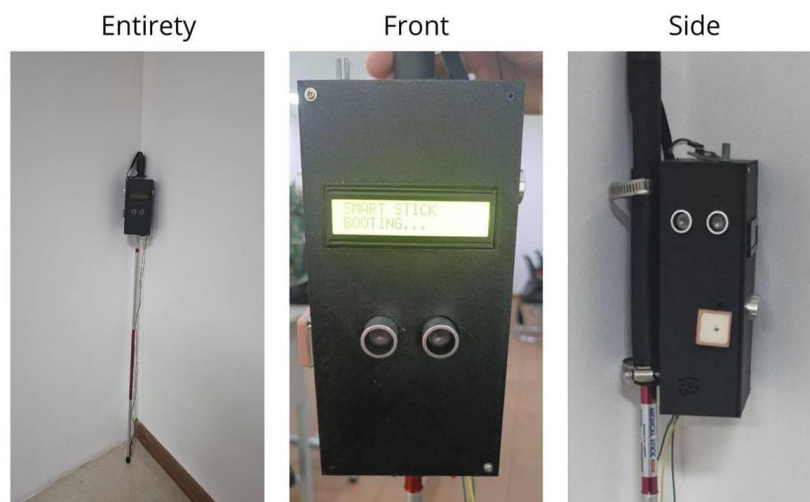
Figure 3. Prototype of the ESP32-Based IoT Smart Cane
