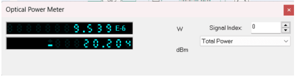
Figure 5. Optical Power Measurement Results on the Receiver Side (ONT1)
