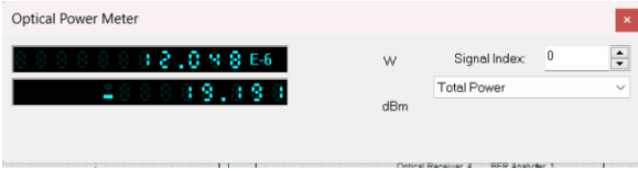
Figure 6. Optical Power Measurement Results on the Receiver Side (ONT2)
