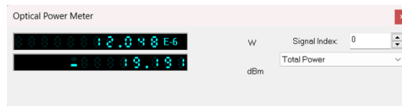
Figure 6. Optical Power Measurement Results on the Receiver Side (ONT2)
