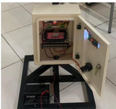
Gambar 1. Kontrol Monitoring Panel Surya
