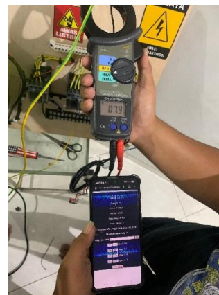
Figure 5. Measurement Comparison Process with Clampmeter
