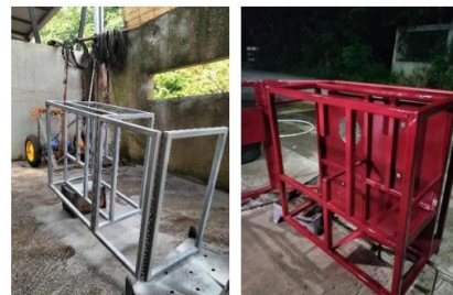
Figure 2 illustrates the bare frame, designed to hold all internal systems in place
