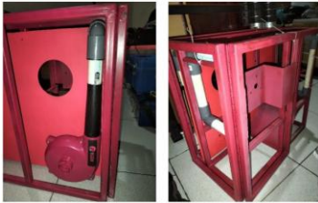
Figure 4 depicts the blower-based drying system integrated within the IHC.
