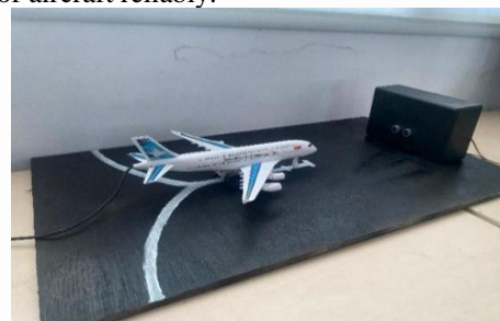
Figure 3. Actual Setup of The Sensor and Nodemcu ESP32 On A Mock-Up Aircraft
