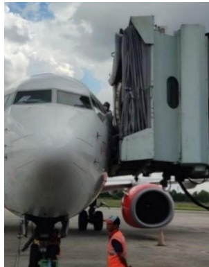
Figure 1. Damage to the passenger boarding bridge canopy
