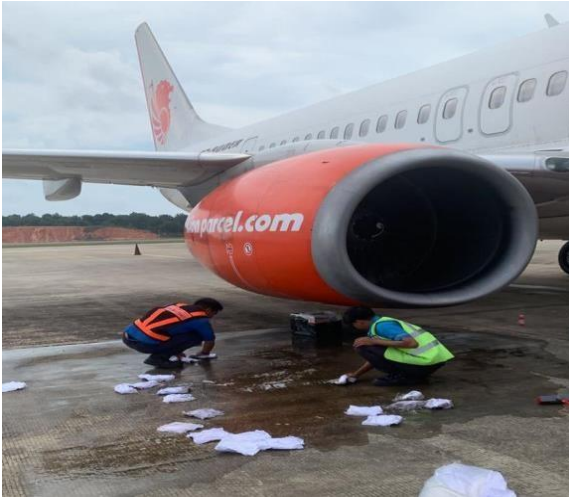
Figure 6. fuel/oil spill from an aircraft engine
