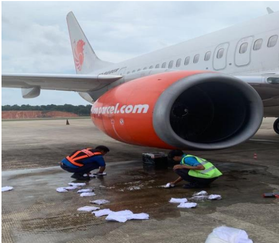
Figure 6. fuel/oil spill from an aircraft engine
