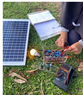
Figure 5 Current and Voltage Testing of Solar Cells using Avometer
