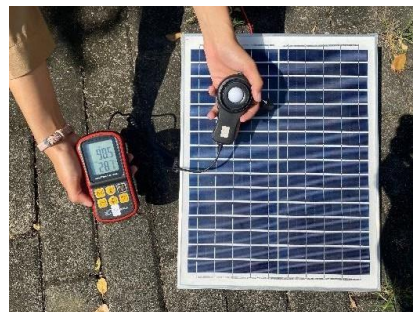
Figure 4 Solar Panel Testing with Luxmeter
