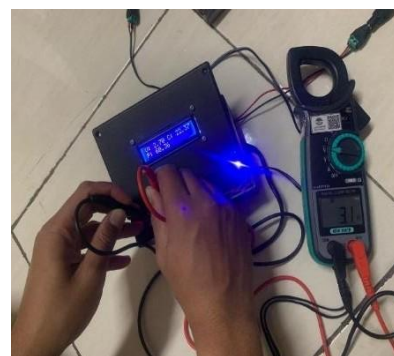
Figure 12 INA219 Sensor Testing
