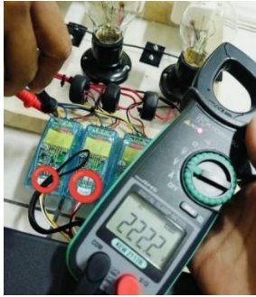
Figure 25. PZEM 004T Testing
