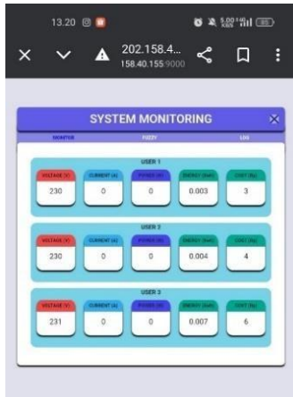
Figure 19. Monitoring system webserver view
