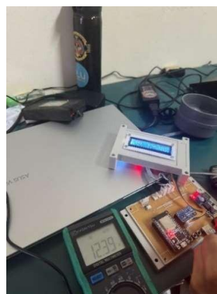
Figure 3 Testing of Buck Converter LM2596
