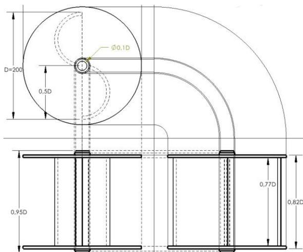
**Figure 1.** Design Turbine Savonius
