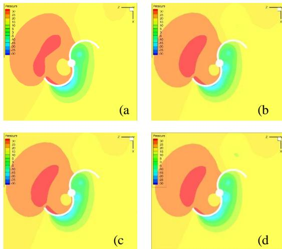
**Figure 7.** Comparison of static pressure contour at 30° angle a) conventional turbine b) turbine with roughness 120 c) ) turbine with roughness 180 d) turbine with roughness 320
