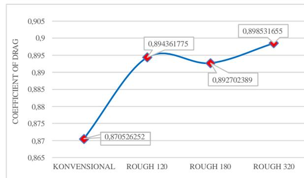
**Figure 6.** Average coefficient of drag graph Based
