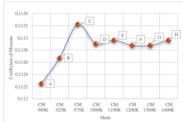
**Figure 3.** Numerical simulation independence grid with moment coefficients ( $C_m$ )
