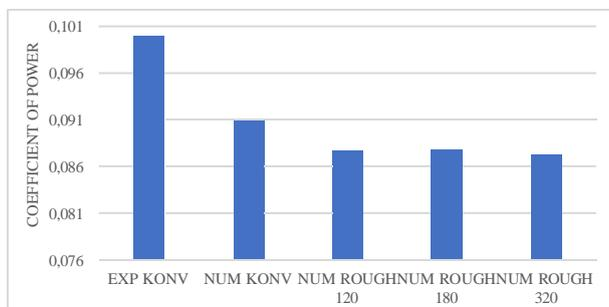
**Figure 5.** Comparison Chart of coefficient of power of experimental and numerical test results
