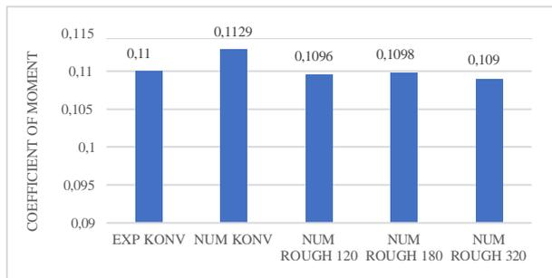
**Figure 4.** Comparison Chart of coefficient of moment of experimental and numerical test results
