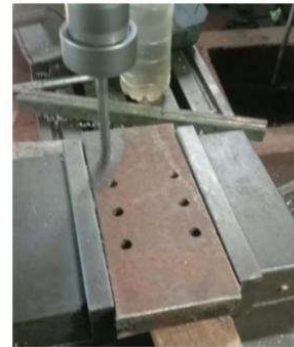
Picture 06. Drilling process
