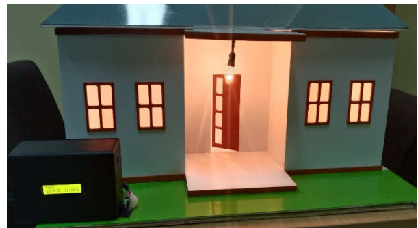
Figure 4 Conditions of the PIR Sensor Detecting Objects Source : Author's Work
