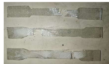
Figure 5. Specimen Test Results (0°,90°)
