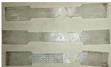
Figure 3. Specimen Test Results (0°,45°)
