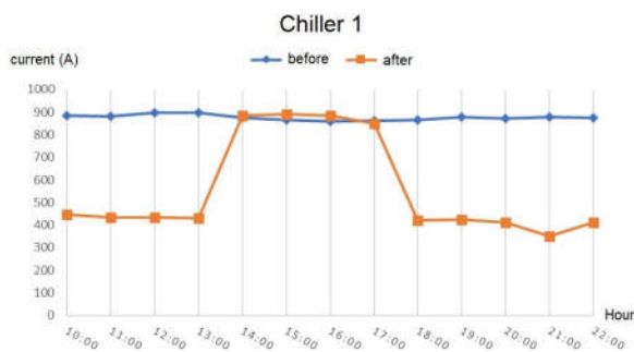
Figure 4. Current of Chiller 1
