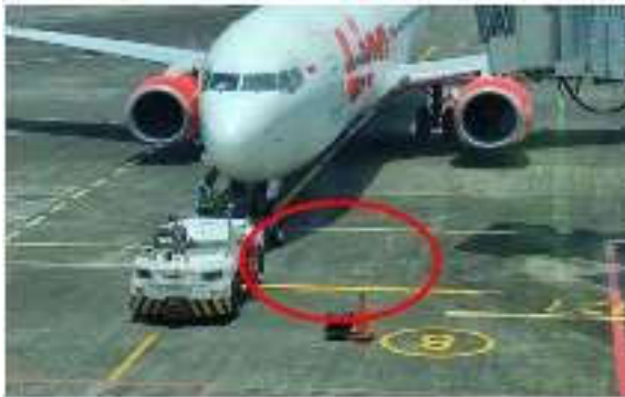
Figure 3 Parking of B737-900 aircraft does not match the actual stop line
