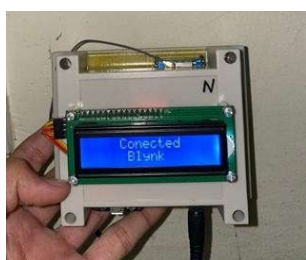
Figure 4.4 Testing the lora module at a distance of 5,100M
