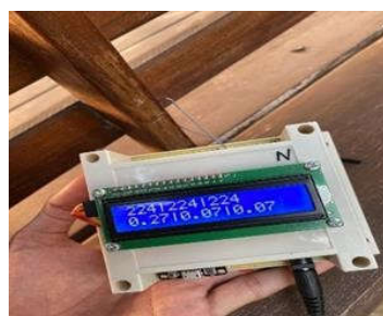
Figure 4.1 Testing the lora module at a distance of 1.608 M
