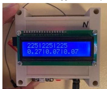
Figure 4.2 testing the lora module to a distance of 3.167 M
