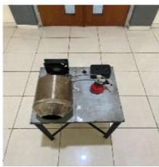
Figure 5. Top view of the annular can combustion chamber simulation working tool.
