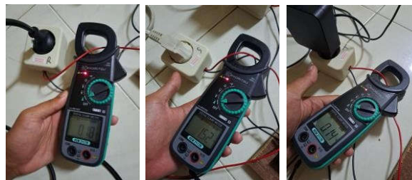
Figure 5 Measurement of Current using a Multimeter
