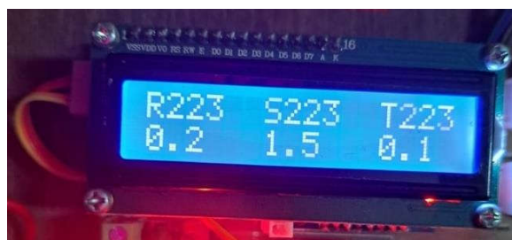
Figure 6 Measurement of Current using PZEM-004T
