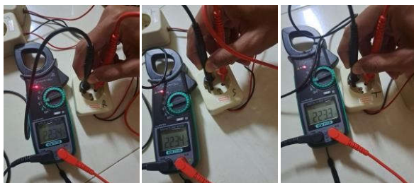
Figure 3 Measurement of voltage using a Multimeter
