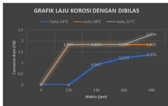
Figure 5. Comparison of corrosion rate with rinsing
