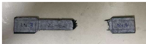
Figure 05. Tensile test of 2 layer (1%) specimen
