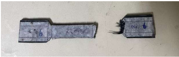
Figure 07. Tensile test of 3-layer specimen (2%)
