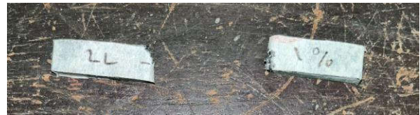
Figure 10. Impact test of 2 layer specimen (1%)
