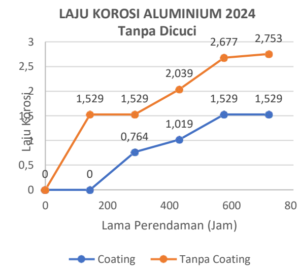
Figure 4. Comparison of Unwashed Corrosion Rate
