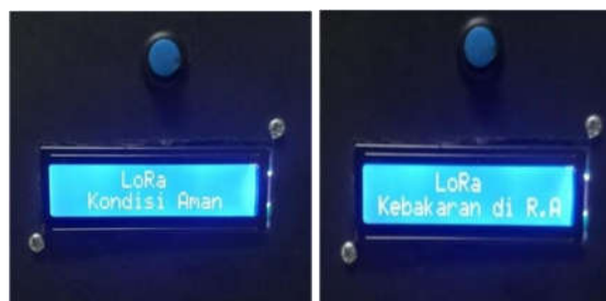
Figure 7. Condition of LoRa Receiver in Standby and active Transmitter
