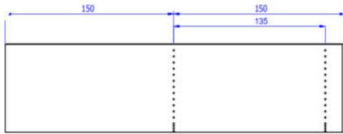
**Figure 4** Pressure tap location on mid span and tip span at all models.
