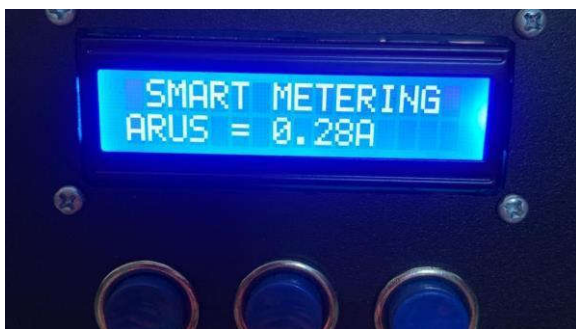
Image 6 LCD display if no power theft is detected
