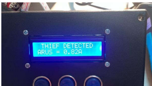
Image 7 LCD display if theft of electricity is detected
