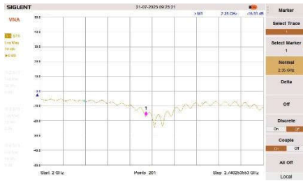
Figure 15 the best circular slot antenna Return Loss measurement results
