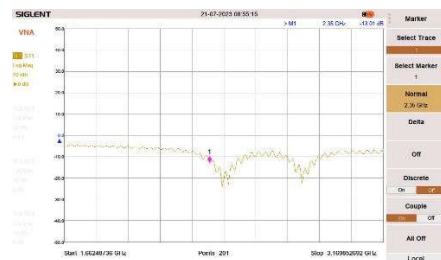
Figure 11 single patch non slot antenna Return Loss measurement results
