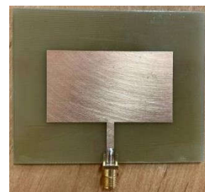
Figure 10 Single Non slot Patch Antenna Fabrication Results
