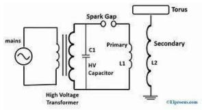
Component Analysis Suite Tesla coil prototype:
