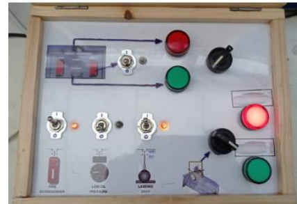
Gambar 15 Foto Uji coba simulator wiring diagram thrust reverser
