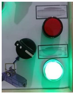
Gambar 13 Selector Switch Thrust Reverser dan Pilot lamp Reverse Retract
