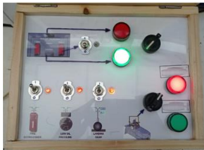
Gambar 17 Foto Uji coba simulator wiring diagram thrust reverser
