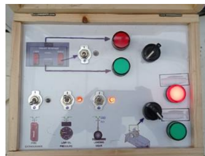
Gambar 16 Foto Uji coba simulator wiring diagram thrust reverser
