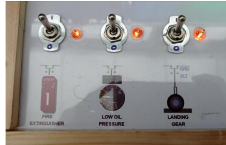
Gambar 11 Toggle Switch Fire Extinguisher, Low Oil Pressure dan Landing Gear
