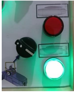
Gambar 13 Selector Switch Thrust Reverser dan Pilot lamp Reverse Retract
