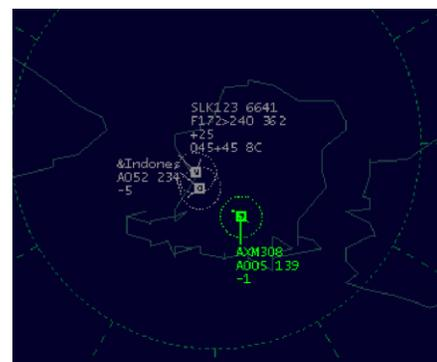
Gambar 11. Hasil Uji coba Rancangan Receiver ADS-B
