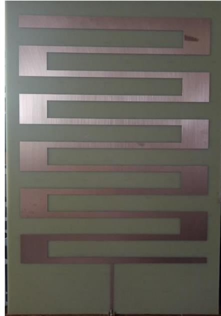
Gambar 9. Fabrikasi Antena mikrostrip meander-line  $\frac{1}{2} \lambda$
