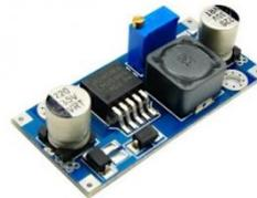
Gambar 11 DC Buck Converter
