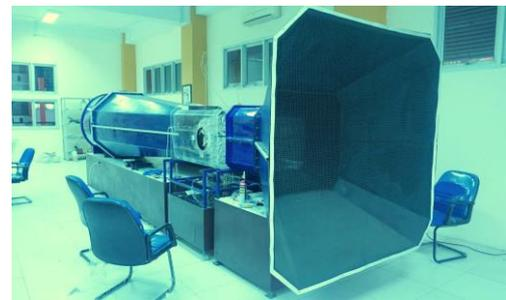
Gambar 3. *Open Circuit Subsonic Wind Tunnel*
