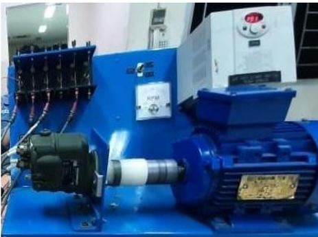
Gambar 3. Magneto Bench Tester
