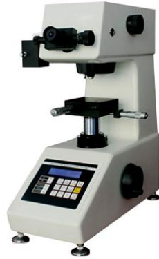
Gambar 3. Mesin uji kekerasan Vickers Digital Micro TH716
