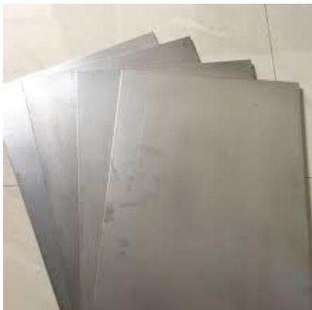
**Gambar 4** Material Titanium paduan (6AL4V)
