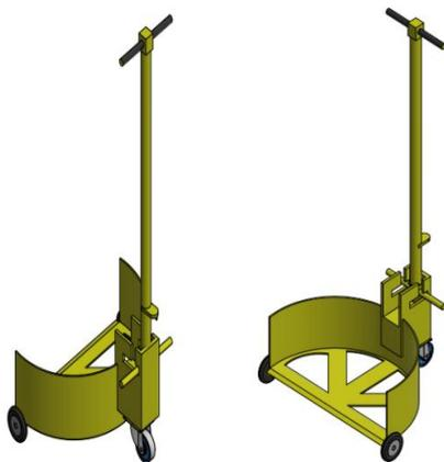
Gambar 2 Desain 3D Trolley Drum Fuel
