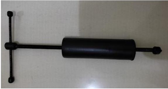
Gambar 3 Special Tool Rocker Shaft Puller
