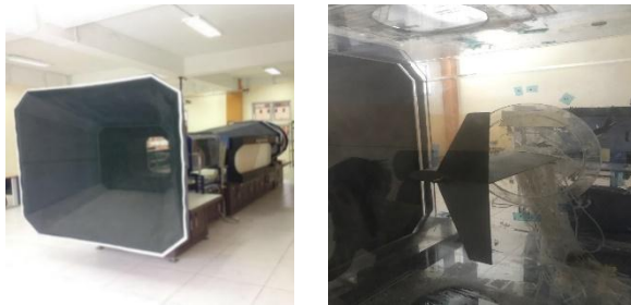
Gambar 3.6. Wind Tunnel Open Circuit Airflow WT-60
