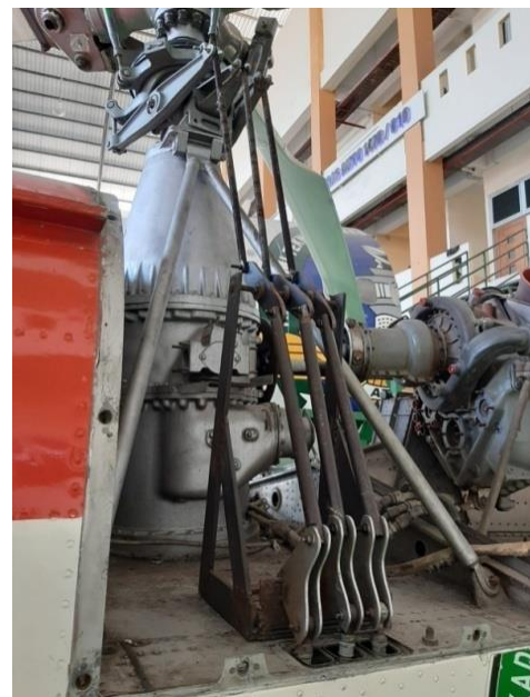
Gambar 4.8 Rangkaian control rods lama
