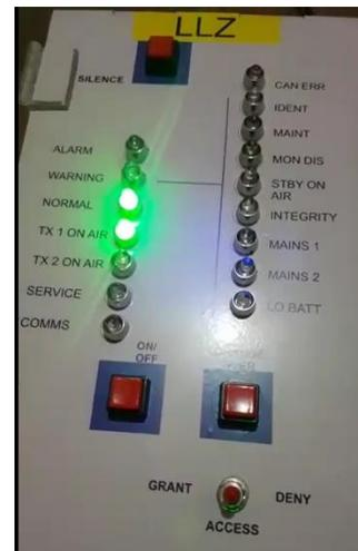
Gambar 12 Indikator Prototype Localizer
