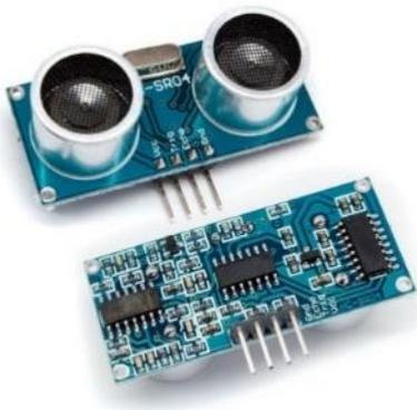
Gambar 4 Sensor Ultrasonik
